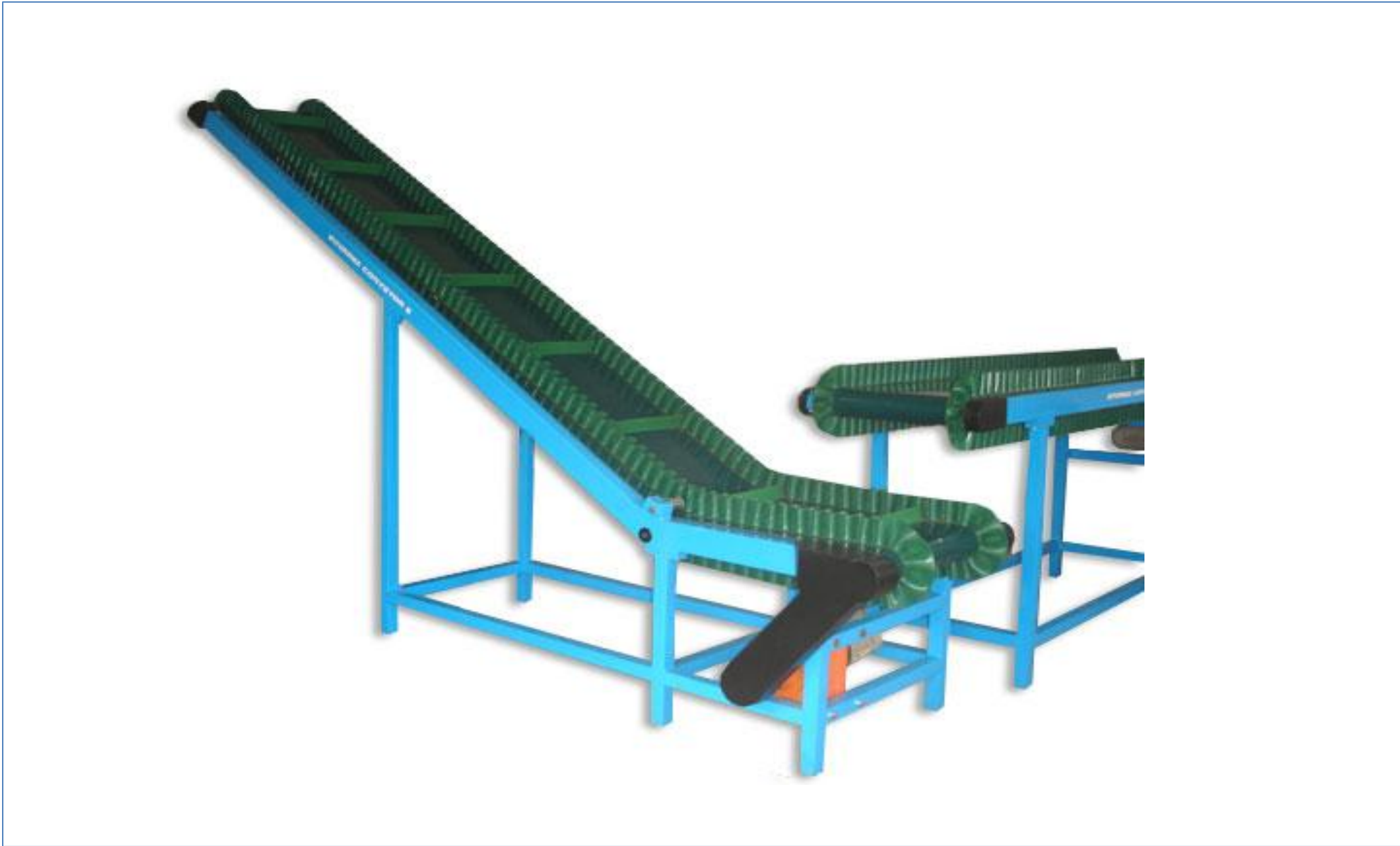
Belt conveyor for unloading hot rubber compound
